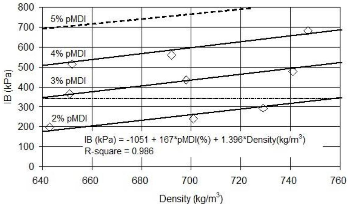
**Fig. 5.** The internal bond (IB) strength of oriented structural straw board as a function of resin content and panel density
