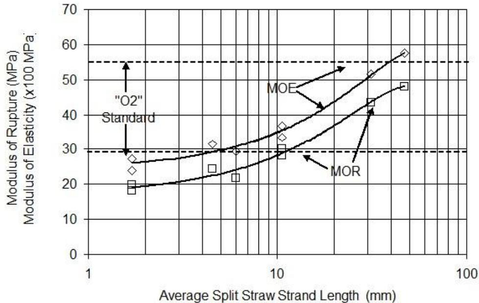
**Fig. 3.** Effects of straw strand length on the modulus of elasticity (MOE) and the modulus of rupture (MOR) of the boards
